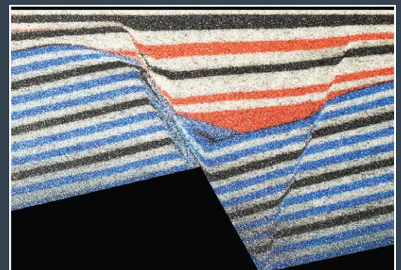
Analogue model showing faulted hanging wall talus wedge
