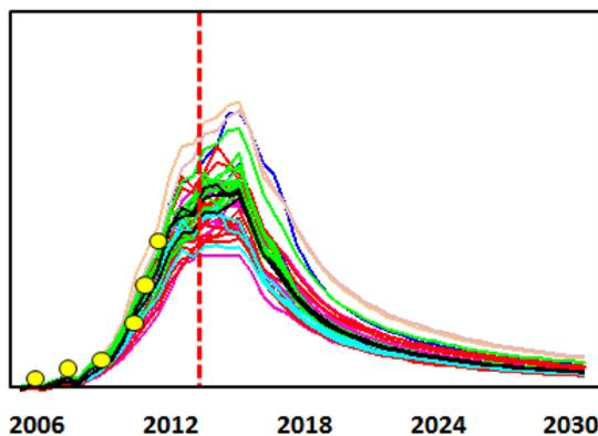
*Simulated production rates for multiple geological models which all match past production data (yellow dots) but lead to different forecasts and hence different optimisation and development strategies.*
