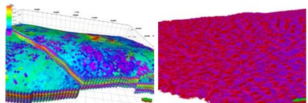
*Example well placement in a fracture reservoir model with matrix permeability (left) and fracture network (right)*
